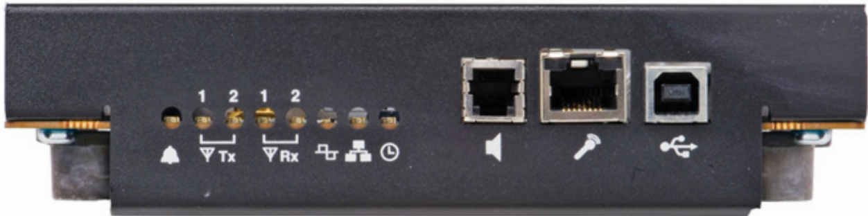
Figure 3-1 Front Bezel LEDs and Connectors
