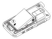
2 To attach battery cover, align it in place and slide the battery latch (<sup>(A)</sup>) until it snaps into place. Slide battery latch into lock position.
